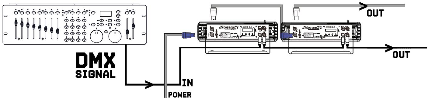
**CAUTION!** At the last unit, you must close the DMX line with a terminating resistor. Take an XLR connector and solder a 120 Ohm resistor between signal (-) and signal (+) and connect it to the DMX output of the last unit in the line.
